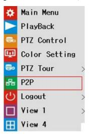
2.setup the IP of LAN, and enable P2P, then it will get an ID automatically, and a pup-up, that says the DVR system must be restarted.
