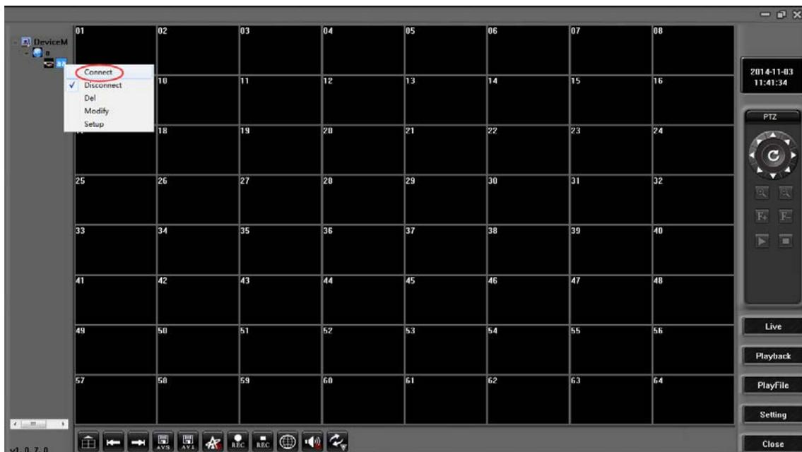
25. Add second device: same way from step 11 to step 24. For step 20 must set First number different to avoid repeating channel display on same channel place. For example No.1 device first display number is 1, channel number is 8, No.2 device first display number should be 9 or more than 9.
